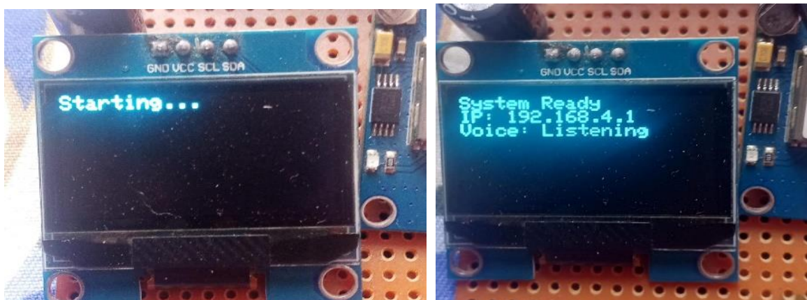
Figure 14: OLED display (a) starting system (b) initializing system.
