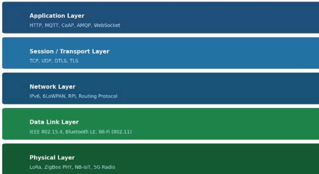
Fig. 4 - IoT Protocol Stack (OSI-Inspired Layered Model)
