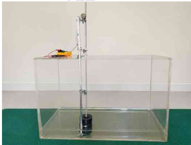
Figure 16: Assembled Power Take-off Column and Guide System Mounted on the Acrylic Wave Tank
