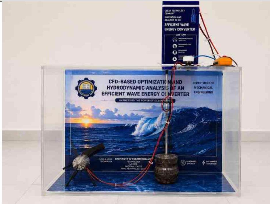
Figure 18: Acrylic Wave Tank used for Experimental Testing of the Fabricated Wave Energy Converter
