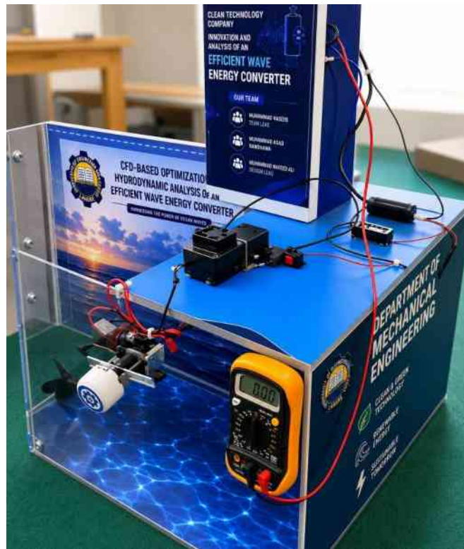
Figure 17: Generator and Electrical Measurement Arrangement of the Fabricated Prototype
