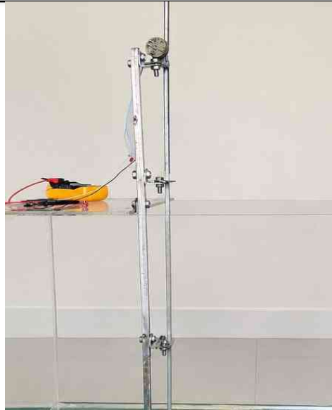
Figure 15: Rack-and-Pinion Power Take-off Mechanism with Aluminum Guide Rail Assembly
