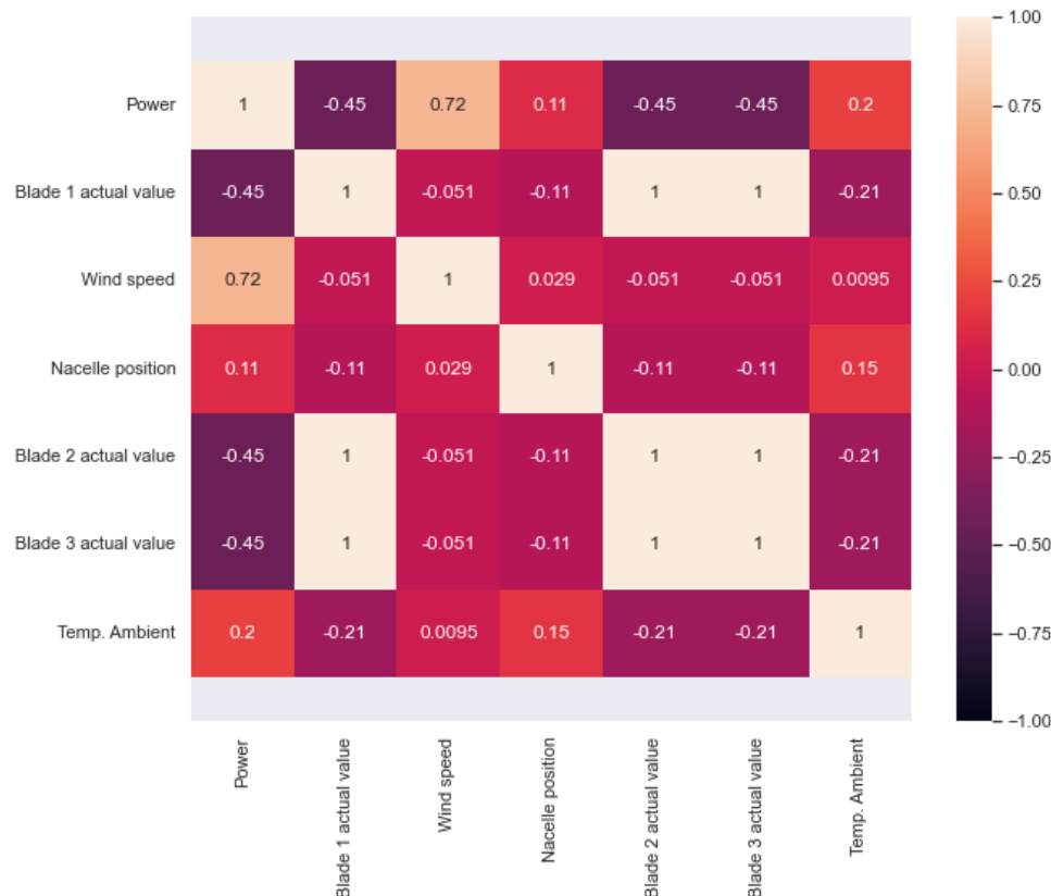
Figure 4: Input features against output power in heatmap correlation
