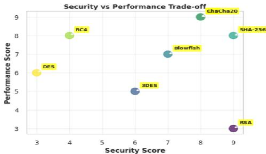
Figure 4: Pareto frontier visualization illustrating the trade-off between cryptographic security strength and performance efficiency across selected algorithms.
