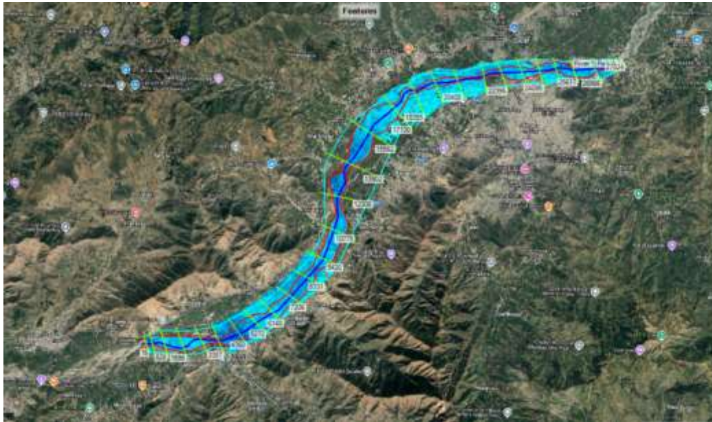
Figure 3.19 Post levee application flood extent, indicating reduced inundation in flood-prone areas
