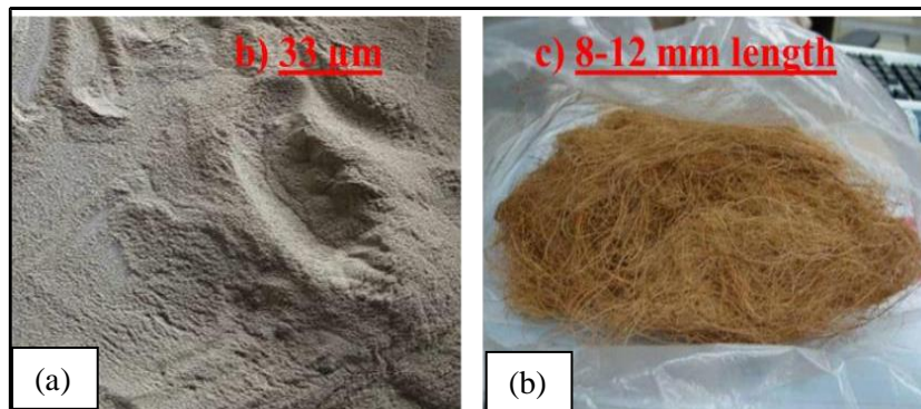
Figure.1 (a) FCBA (Fine coal bottom ash); (b) Coir Fiber
