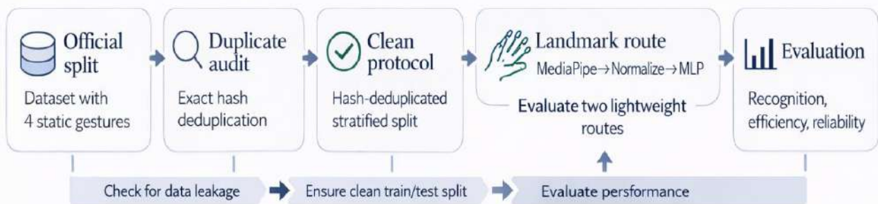
Figure 1. System overview of the leakage-aware benchmark pipeline for the four-command touchless document interface
