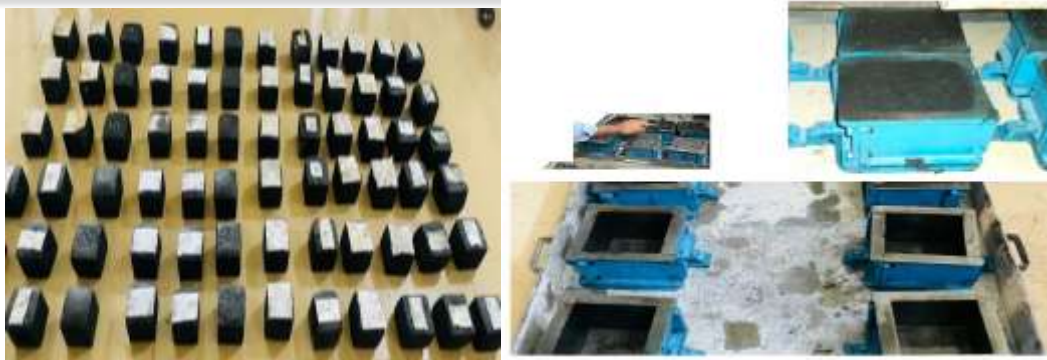
Figure 3 Casting of Specimen
