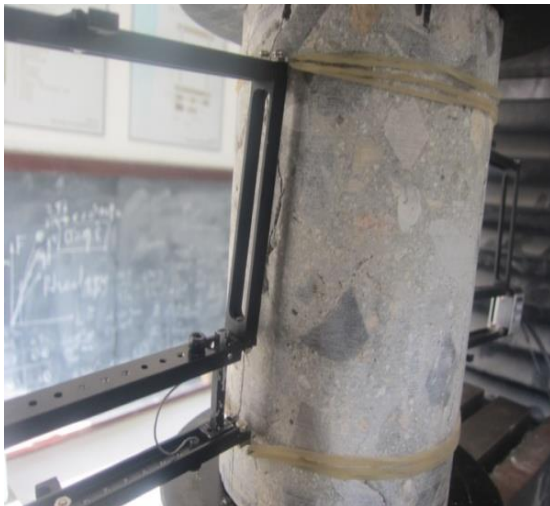
Fig. 17 - OLD4 Specimen cracks propagation
