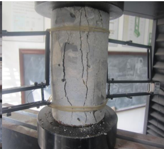
Fig. 14 - OLD3 Specimens failure
