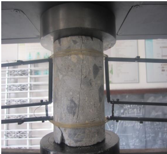
Fig. 13 - OLD3 Specimen crack propagation
