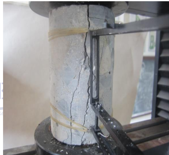
Fig. 18 - OLD5 Specimens cracks propagation
