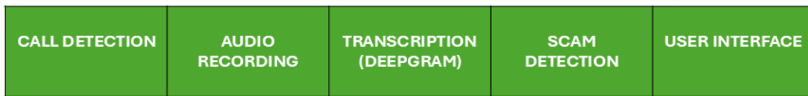
Figure 1: Modular system architecture for real-time scam call detection, illustrating the sequential pipeline from Call Detection through Audio Recording, Deepgram Transcription, Naïve Bayes–based Scam Detection, and the User Interface Alert module.
