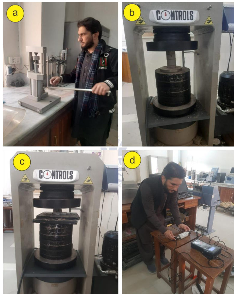
Figure 3: Photographs showing various geotechnical tests. a) showing Point Load Test of the core samples; b) showing Unconfined Compressive Strength test of the core samples; c) showing Unconfined Tensile Strength test of the core samples; e) showing Ultrasonic Pulse Velocity test of the core samples.
